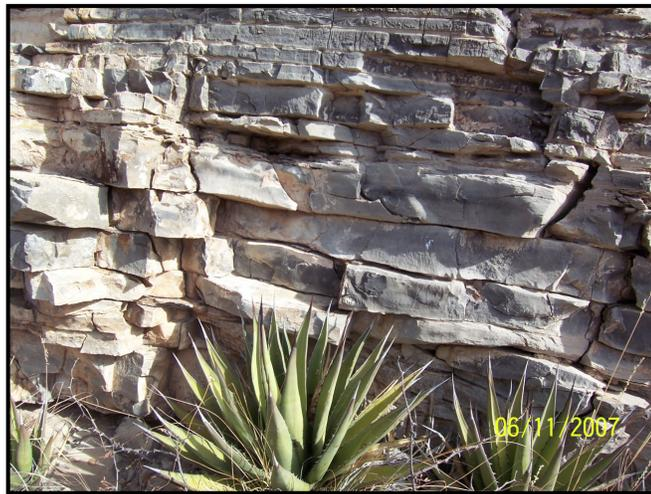
Figure 1-1: Alternative thin layers may result in anisotropic structure.
