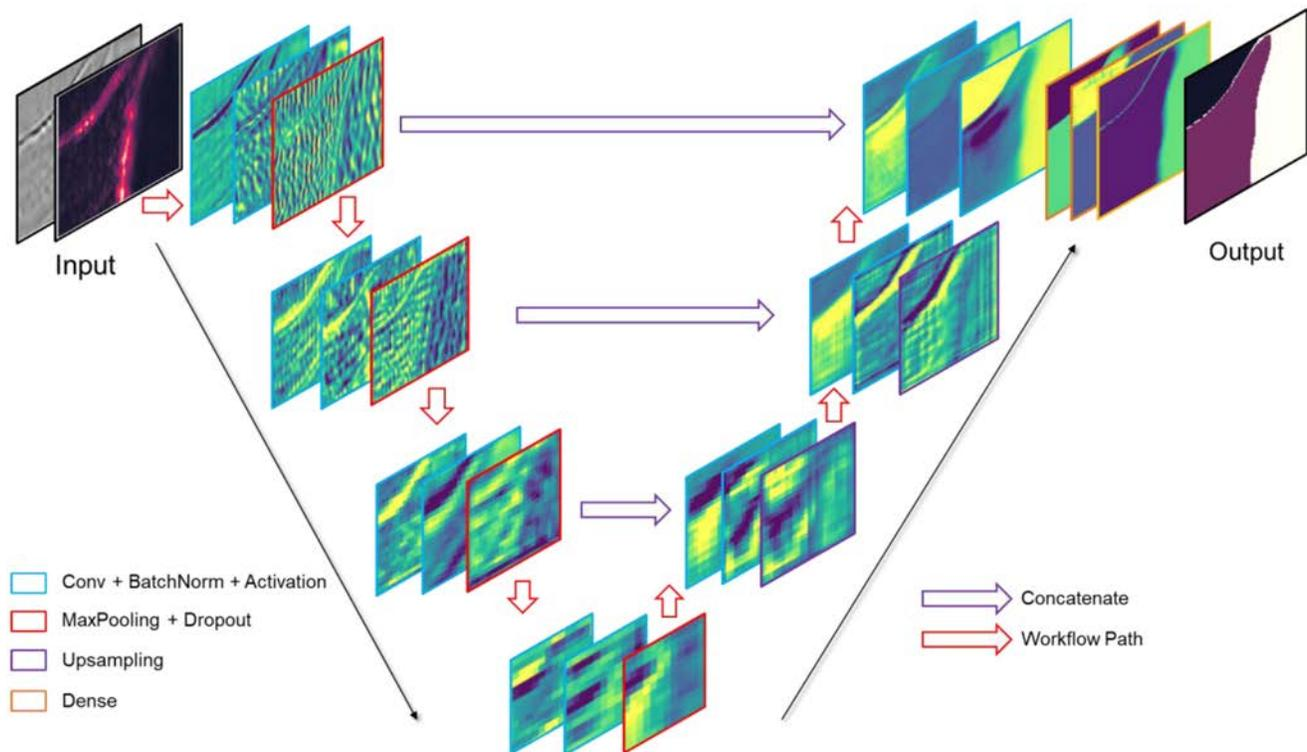
Figure 3—The deep convolutional network with saliency map. The inputs are seismic and saliency maps, the output is classified segments. Each layer shows different feature maps at different depths of the neural network.
