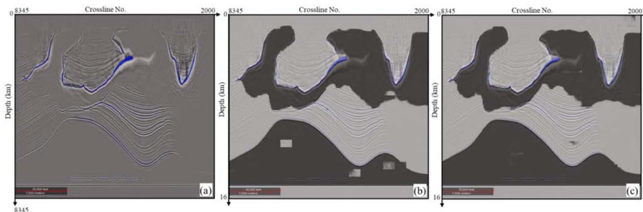
Figure 4—The results of binary salt classification. (a) The original seismic; (b) Prediction by seismic-only model; (c) Prediction by seismic-plus-saliency-map model. Notice that some areas misclassified in deep salt are corrected in (c).
